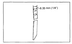
Insert the blade into the blade holder as far as it will go. Make sure that the end of the blade shank reaches the bottom of the inner slit and tighten the bolt securely with the hex wrench.
